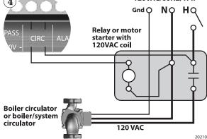
Figure 15 Circulator wiring terminal strip (see Figure 11 for location) — Also see the wiring summary illustrations on the next pages)
