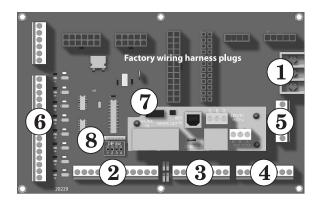
Figure 2 120VAC power service terminals on electrical connection board — See Figure 15 for location of the power terminal strip
